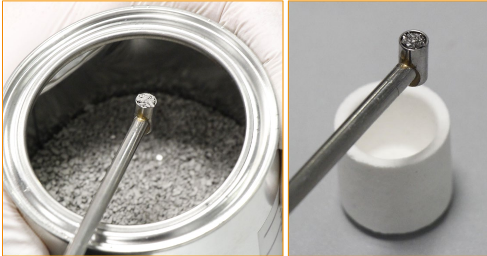
Application of tungsten with spoon (part number 23113)
